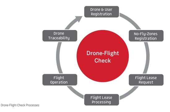
The key of the Drone-Flight-Check solution is to dynamically link the registration database and the individual flight lease requests of the users to an area database where all no-fly-zones or limited fly-zones are centralized and updated. This shall for example prevent a user to fly into a temporary no-fly-zone or enable only specific categories of drones/ users to fly into a specific area.
